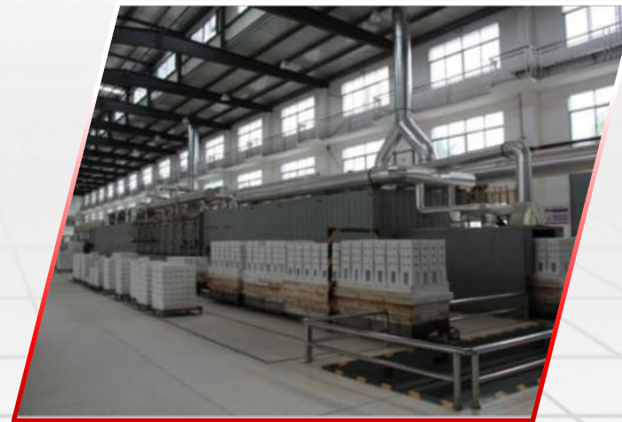
Tunnel kiln (32m)
