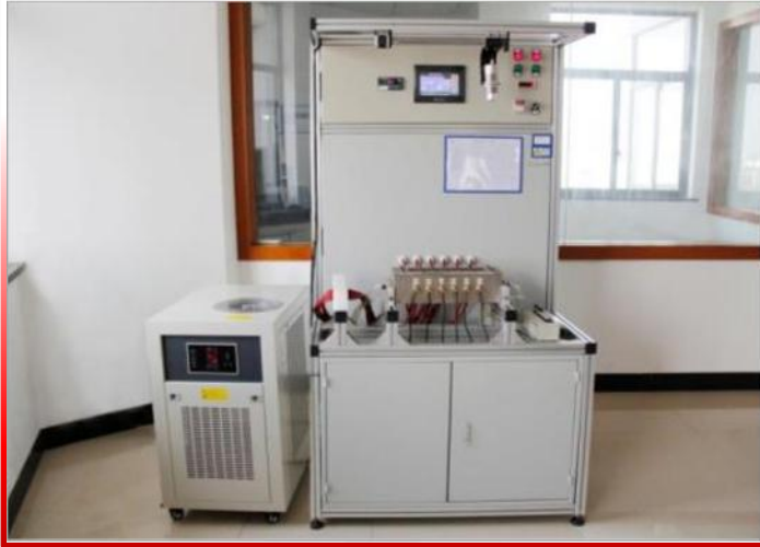
High voltage dielectric performance test equipment
