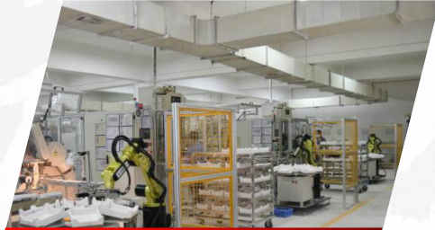
Fine Ceramic Automatic Production line by Robots
