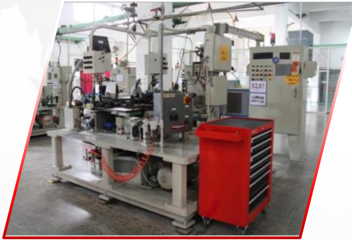
laser welding equipment (precious metal electrode)
