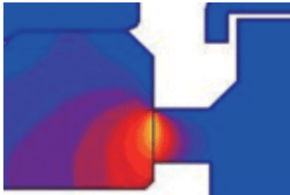
Rendered image of thermal and structural analysis of mechanical seal face materials
