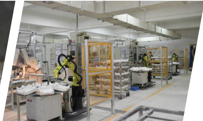
Fine Ceramic Automatic Production line by Robots
